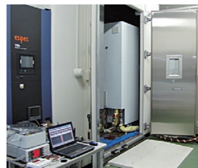
Environmental durability test using a constant temperature room
