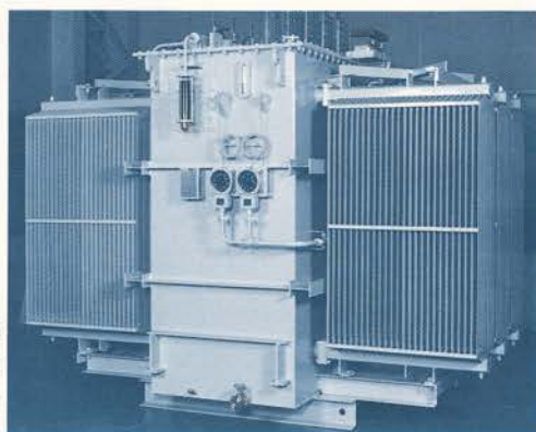
スコット結線油入自冷式炉用変圧器 (Scott Connected Oil Immersed Self Cooled Furnace Transformer) 3/2φ 5000kVA 6000/340V
