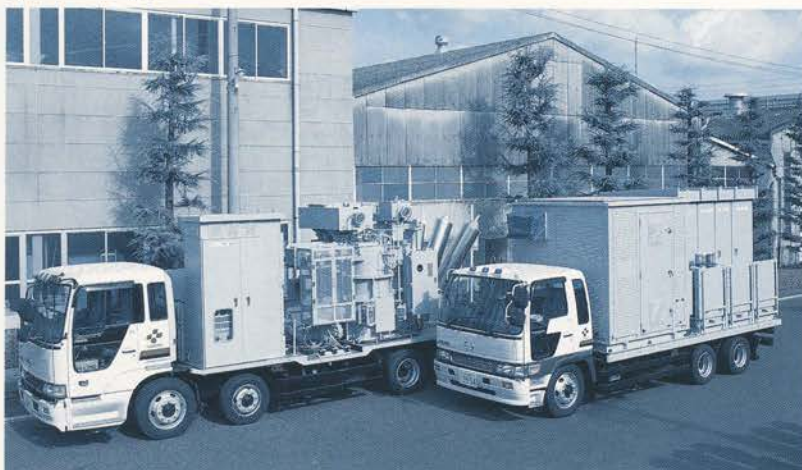
移動用変電所 (Mobile Type Transformer Substation) 10MVA 66/6.9kV TR.5Switchgear
