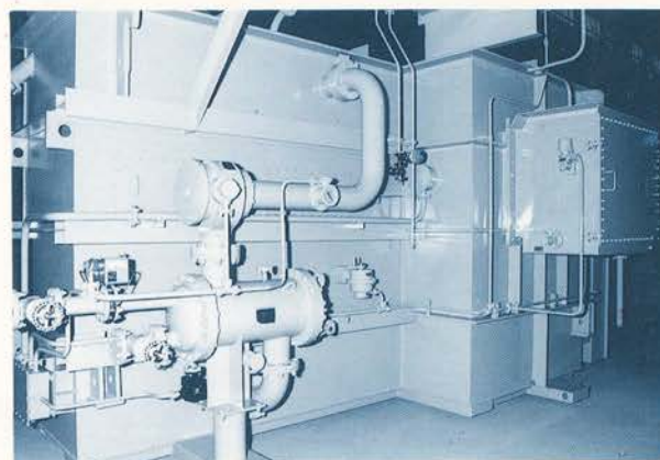
送油水冷式負荷時タップ切換サイリスタ用変圧器 (直流リアクトル内蔵) (Oil Immersed Water Cooled Rectifier Transformer With On-Load Tap-changer and DC Reactor) 6490/9170kVA 6600/242~82V
