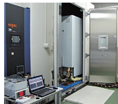
Environmental durability testing using a thermostatic chamber
