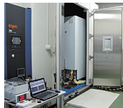
Environmental durability testing using a thermostatic chamber
